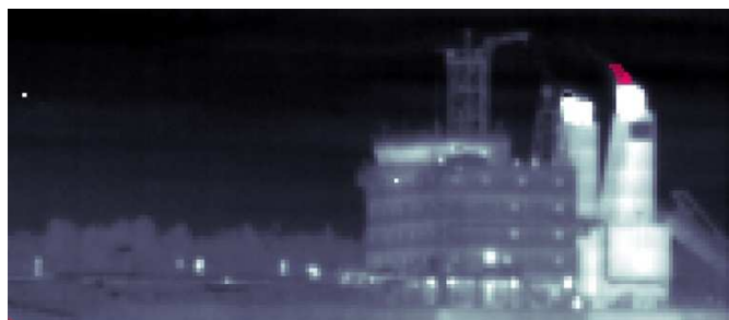
Figure 2. SO 2 detection of a moving ship. The ship is moving eastward (toward the left) on the Saint-Lawrence seaway.
